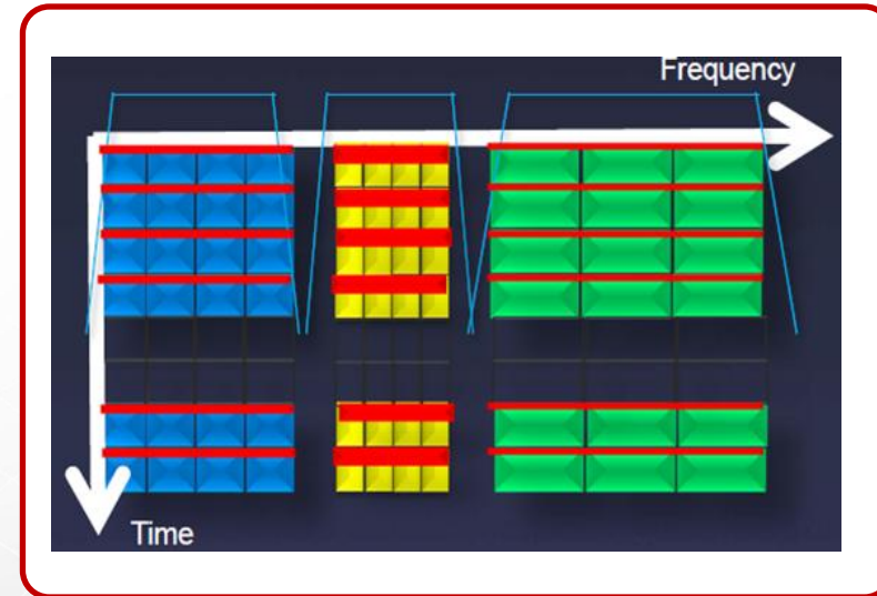
Different Cyclic prefix for each specific sub-band
