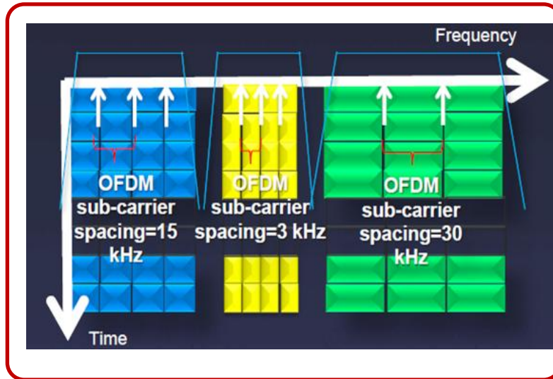
Co-existence of waveform with different OFDM primitive
